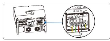
Step 4 Lock the AC OUTPUT terminal shell back to the original position, Stretch all the lines on the AC end naturally and then tighten the plug.
