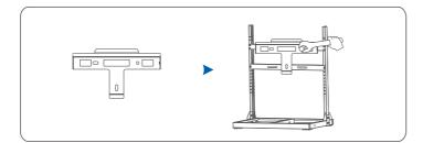
Step 2 Mount the inverter on the rear panel and keep them aligned with each other.
