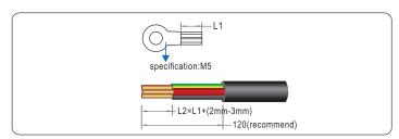
Step 2 Insert the exposed core wires into the crimp area of the OT terminal and crimp them using hydraulic pliers. Wrap the wire crimp area with heat shrink tubing or PVC insulation tape.
