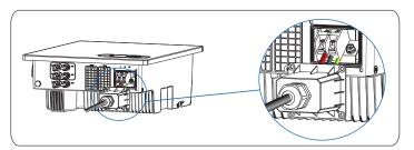
Step 4 Rout AC output cables to L, N and PE on the AC terminal block respectively, and tighten them using screw driver to a torque of 1.5N.m.
