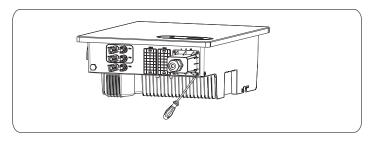
Step 6 Use a torque wrench to tighten the locking cap on the AC cable to a torque
