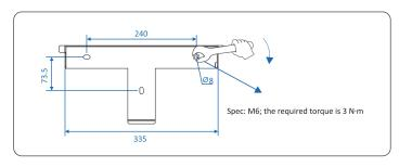
Step 6 Mount the inverter on the rear panel and tighten the screws at both sides.
