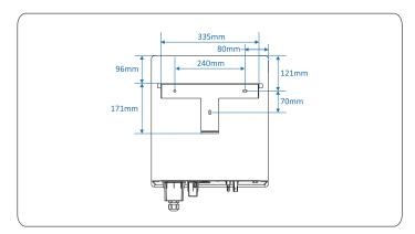
Step 3 Level the hole positions using a level, and mark the hole positions using a marker.
